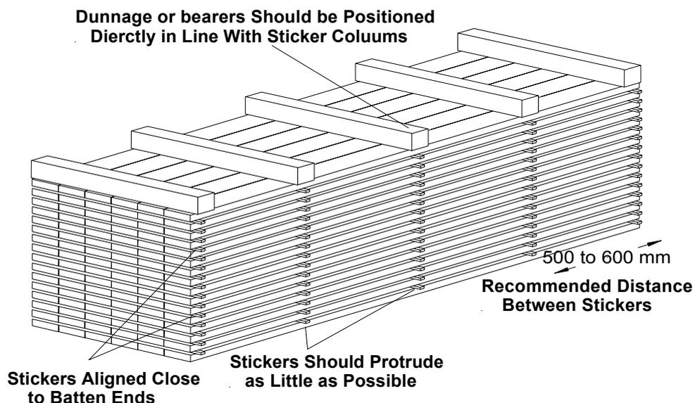
To minimise distortion developing during the drying process, the stickers must be positioned at regular intervals across each layer of battens thus providing support to each successive layer. Battens within a parcel are therefore supported by those stickers above and below each layer as shown in figure 1. In turn each parcel is supported by dunnage positioned below each column of stickers, which is supported by the kiln floor or bogie.
