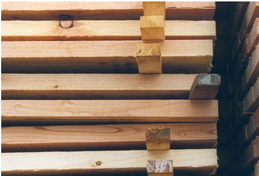
Figure 2b. Sticker Displacement & Alignment Inducing Distortion
