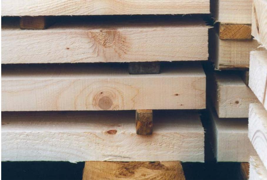
Figure 2a. Incorrect Sticker Alignment & Placement
