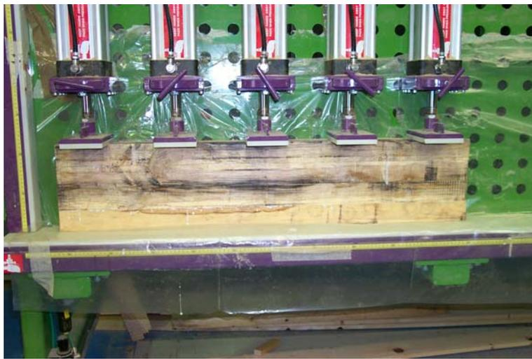
Figure 5. Cut quarter sections being pressed
