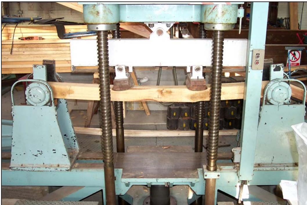
Figure 7. Solid oak beam under test
