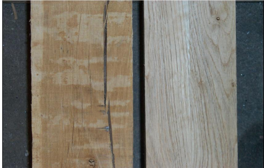
▲ Surface finish of solid and re-engineered oak beam after drying
