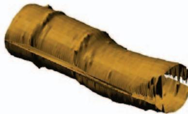
▲ 3D log image processed at BRE using data from a commercial scanner
