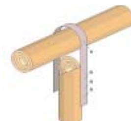
**Round column head/sawn beams connection**
