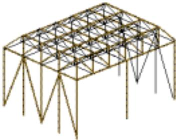
Span: 10x16m, 8x18m typical two ways spanning
