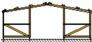
Span: 7.5m; lower eaves height : 2m
