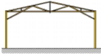
Span: up to 20m; height under knee brace: 4.65m
