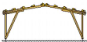
Span: up to 20m; eaves height 3.85m
