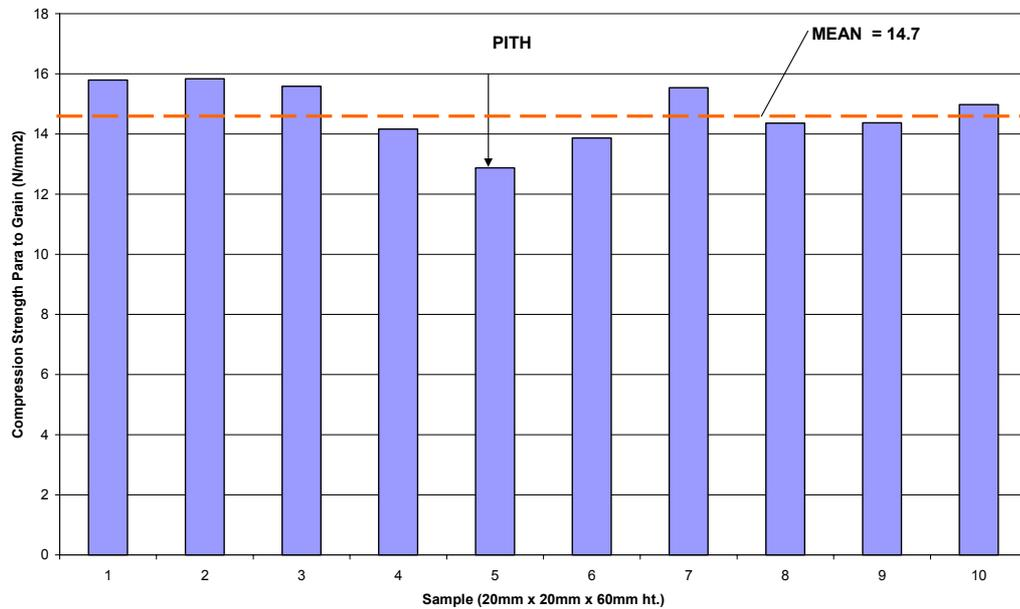
**Figure 13: Compression parallel to grain tests on small scale samples**
