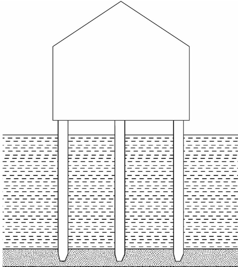
**Figure 1: End bearing piles**
