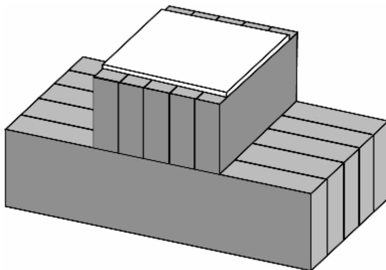
**Figure 15: Column foundation pad (After CWC, 1997)**
