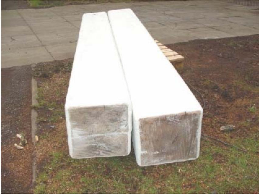
**Figure 8: Impact resistant and highly durable Fibre Reinforced Polymer coated UK grown Douglas fir, for marine borer protection.**
