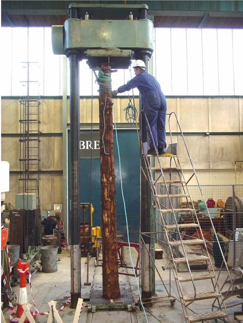
**Figure 11: Axial load test on a Sitka spruce log**
