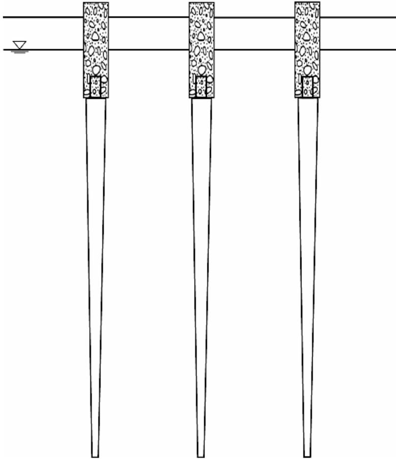
**Figure 2: Tapered friction piles, extended above the water table using concrete sections**
