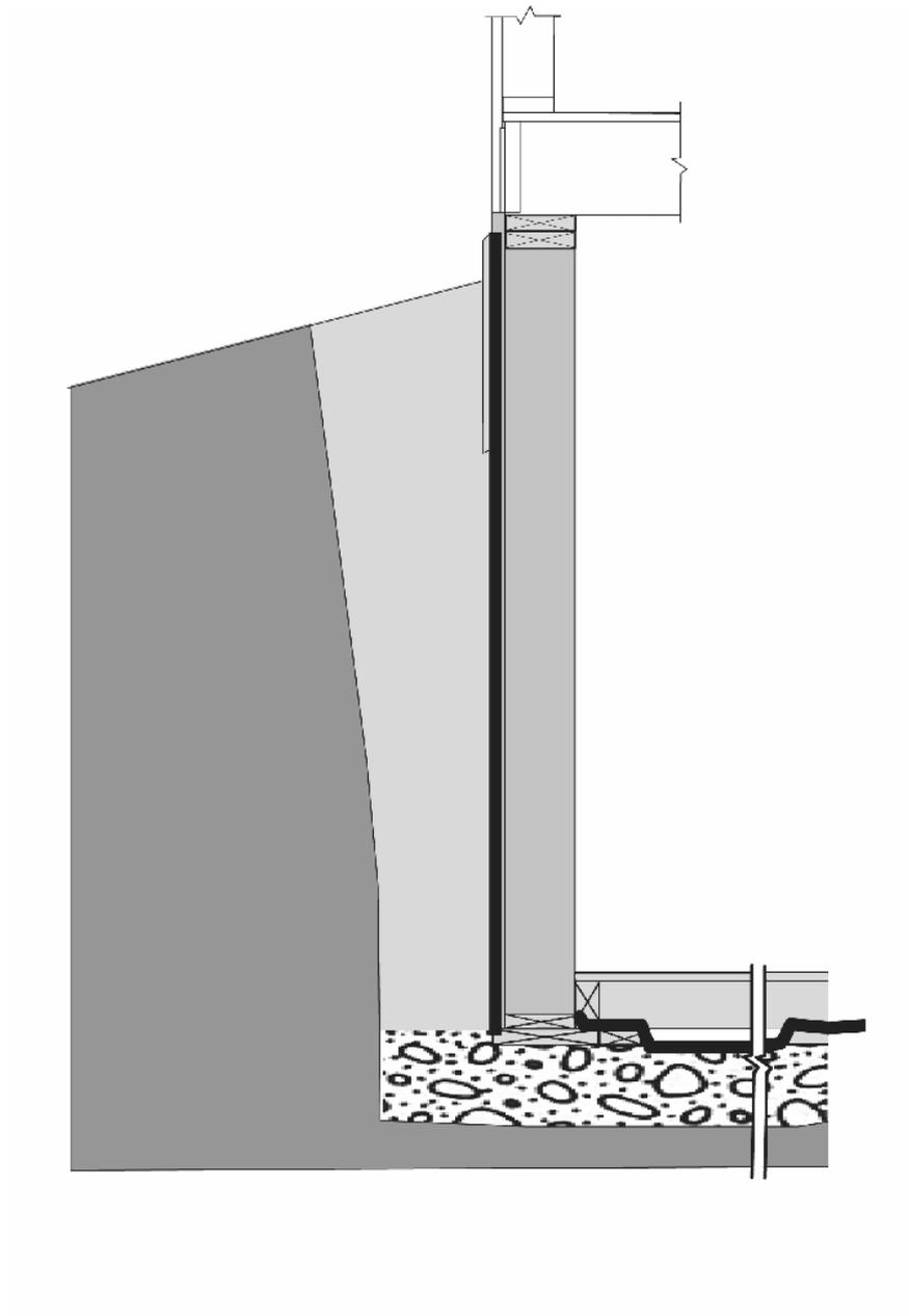
**Figure 14: Basement constructed using Permanent Wood Foundation method
