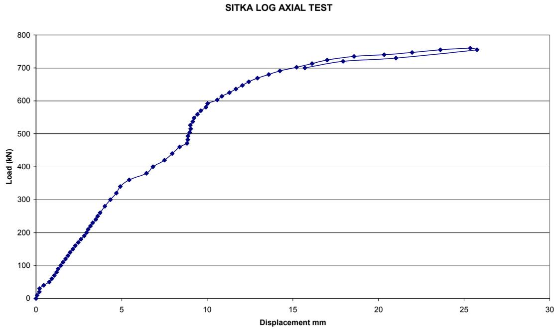
**Figure 12: Axial load test results**
