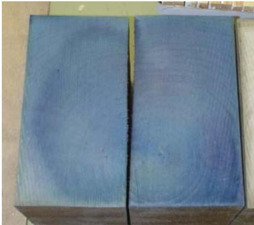
**Figure 7: 150mm square sample of Copper Chrome treated sycamore after cross-cutting and application of an indicator chemical (blue) - showing good penetration throughout the specimen**
