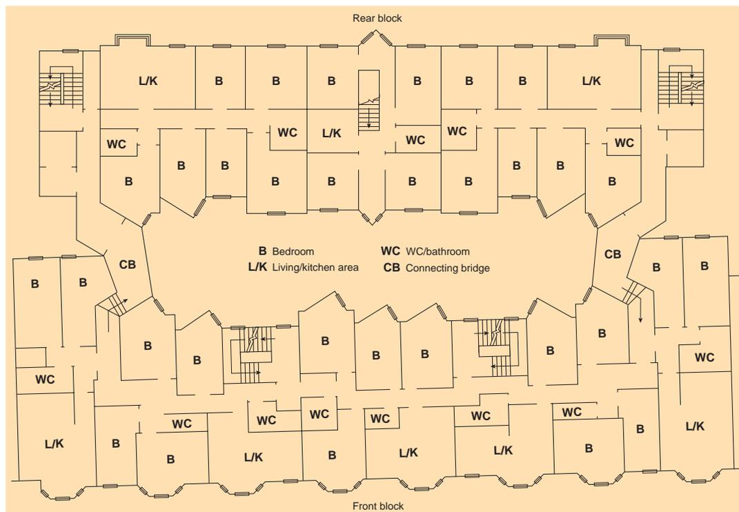
Schematic plan of the new building at first-floor level
