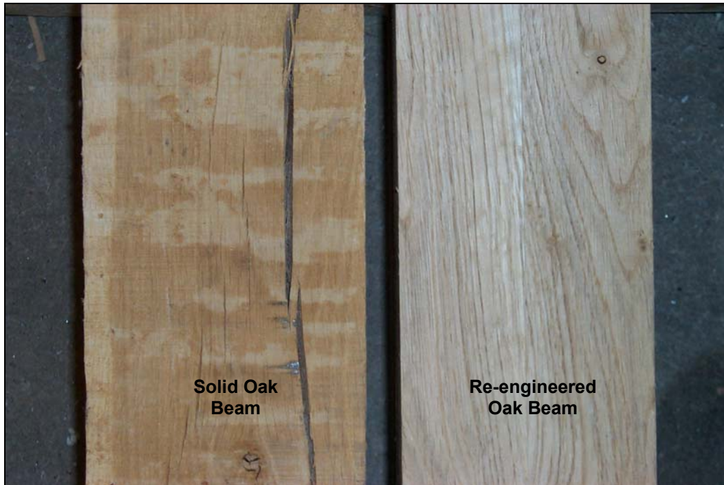
Figure 9. Surface finish after drying
