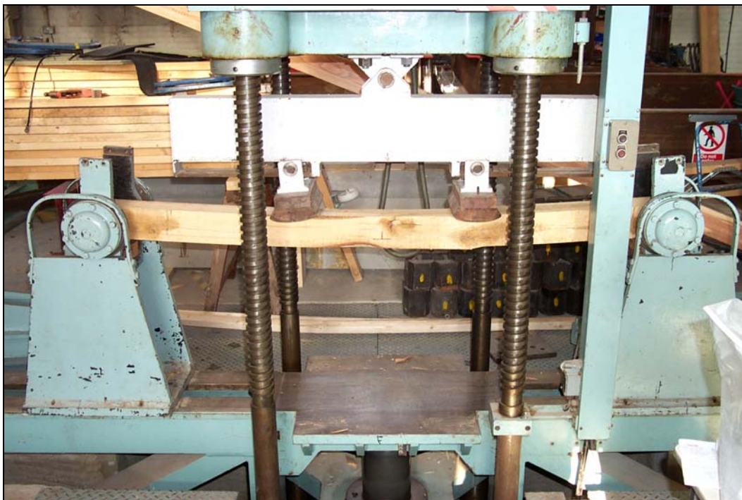
Figure 7. Solid oak beam under test
