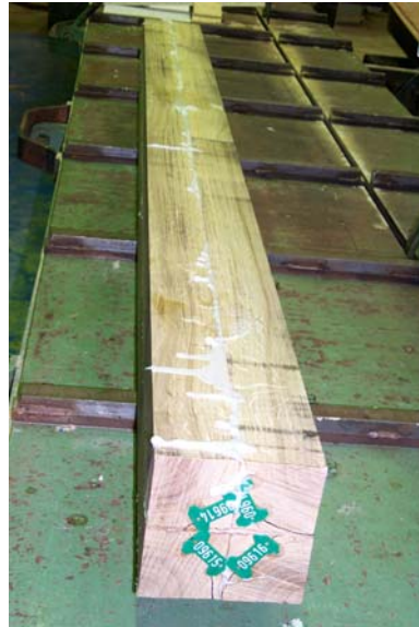
Figure 6. Re-engineered oak beam
