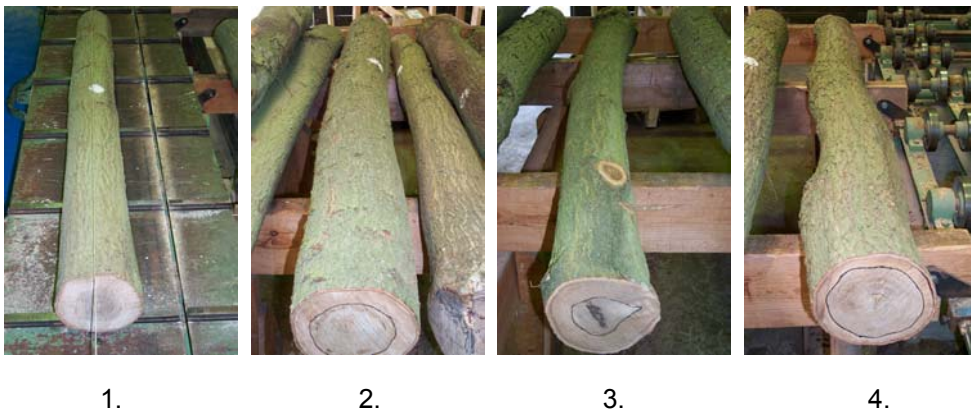
Figure 3. Stem straightness of oak logs categorised as per the Forestry Commission protocol
