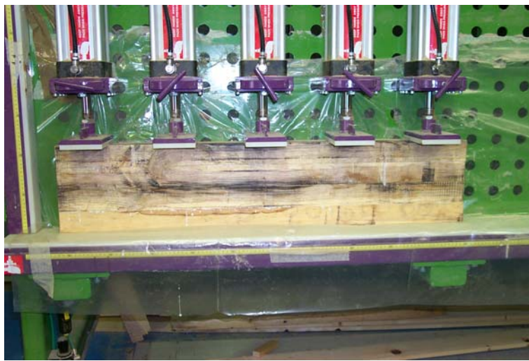
Figure 5. Cut quarter sections being pressed
