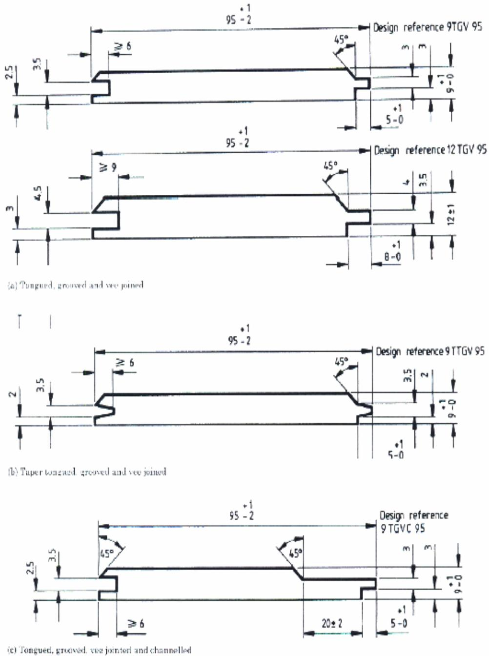
Figure 6: Possible cladding profiled as listed within BS1186-3 (1996).
