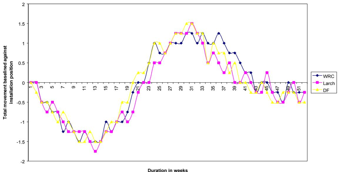
Figure 4. Total dimensional movement to 52 weeks - overlapped panels
