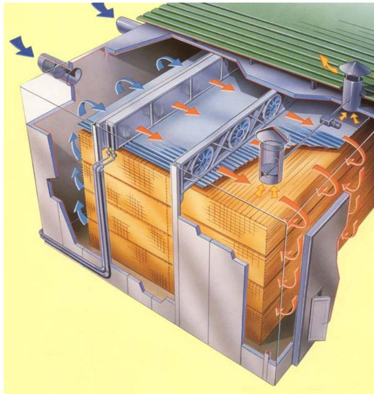
Figure 1. Exploded diagram of a wood drying kiln (over-head fan batch kiln)
