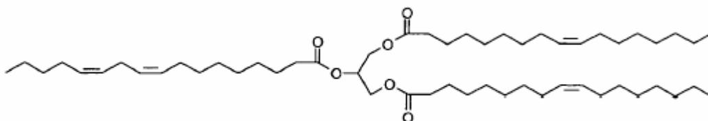
**Figure 5** A triglyceride molecule. Triglycerides are the main component found in natural oils
