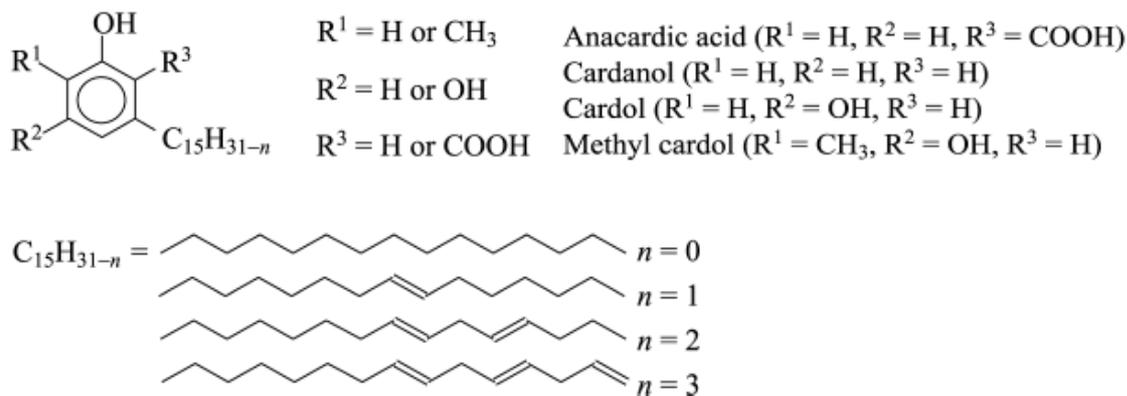
**Figure 4** Components of CNSL.
