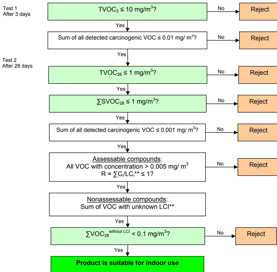
**Figure 6** Schematic overview of German VOC testing procedure for building products
