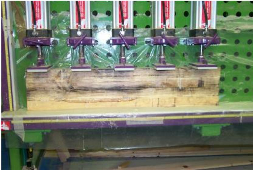
Figure 5. Pressing of cut quarter sections
