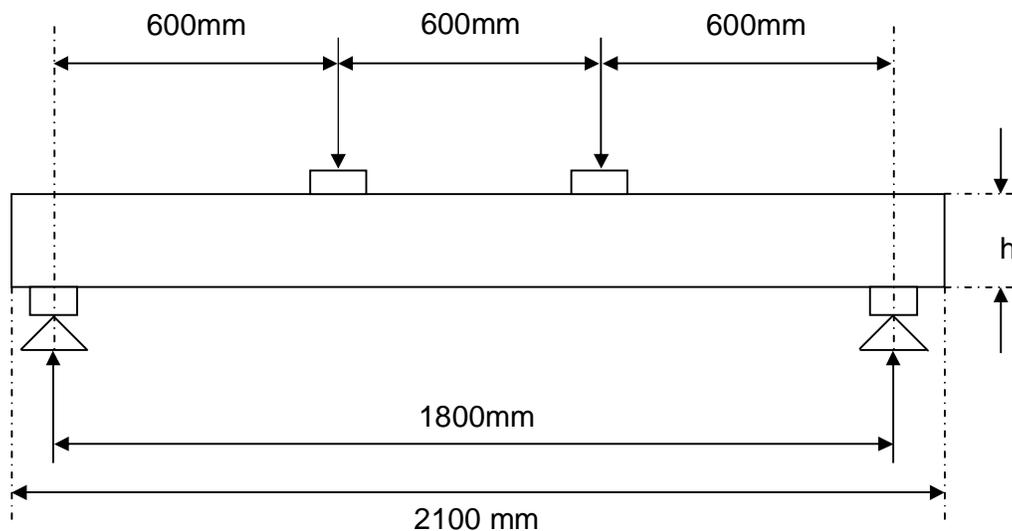
Figure 12. Set-up for four-point bending
