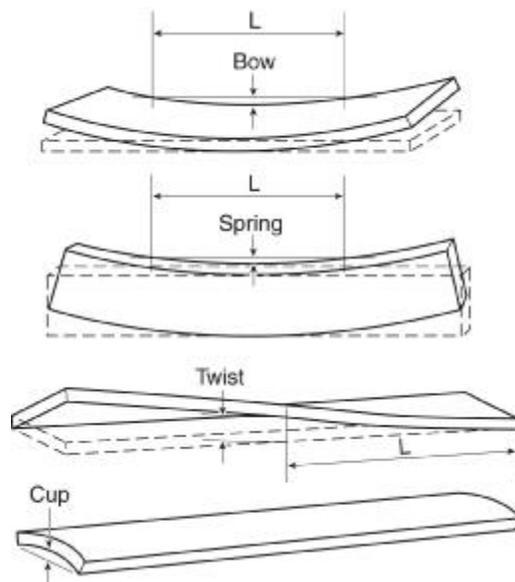
Figure 1. Distortion Types
