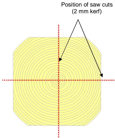
Figure 9. Cut stem into four sections
