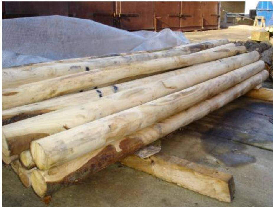
Figure 4. Machine rounded stems
