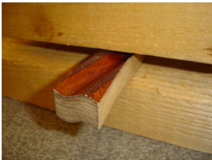
*Figure 6. Laminated and fluted Laonda sticker (courtesy of Sperrholzwerk Schweitzer)*
