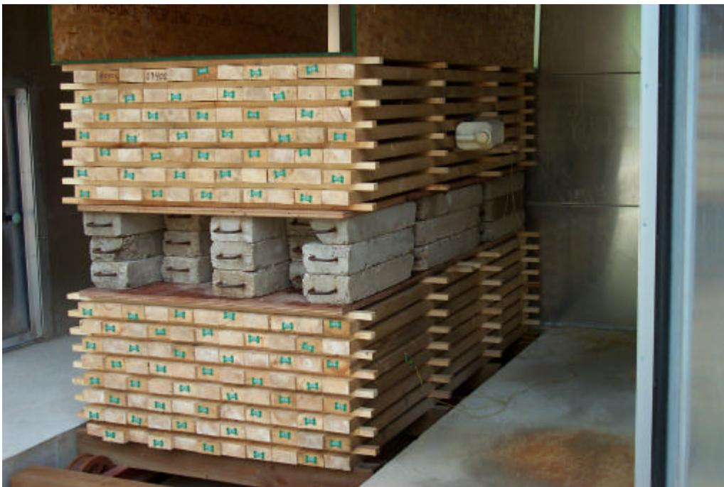
Figure 4. Experimental kiln trial showing loaded and un-loaded material
