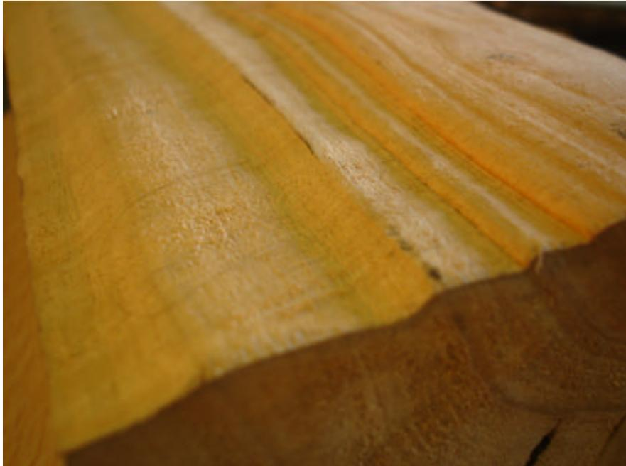
*Figure 11. Batten showing severe collapse*
