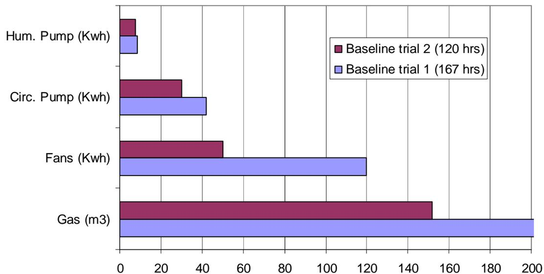
Figure 4. Comparison of energy consumption during the baseline control trials
