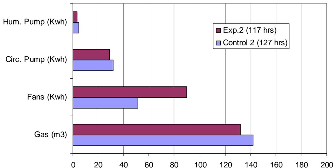
Figure 6. Comparison of energy consumption from trial 2
