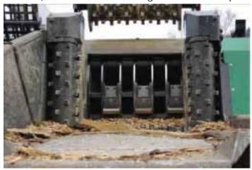
Sharp blades are a must for the production of sharp-edged quality wood chips
