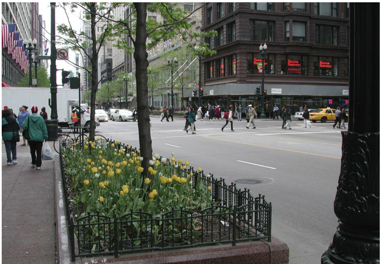
Figure 3 Each tree in a shared planting space of this size could have a crown diameter of no more than 4 m or be subject to annual drought stress without supplemental irrigation according to a computer model (DeGaetano, 2000).
