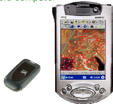
Image 2. iPAQ Pocket PC with satellite images and EMTAC GPS with blue tooth communication.
