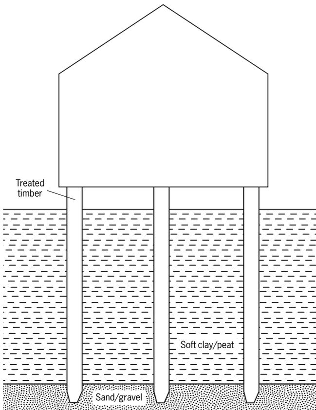
**Figure 1** End bearing piles
