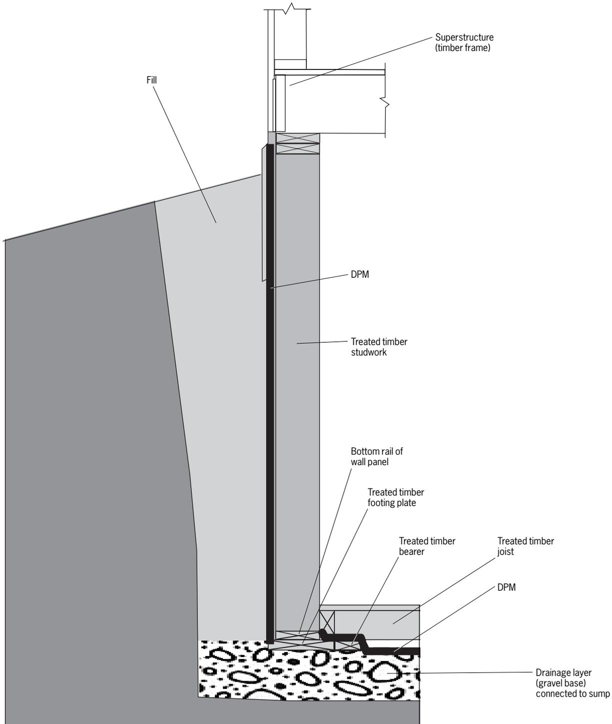
**Figure 6** Permanent Wood Foundation system for a basement (after Canadian Wood Council, 1997)
