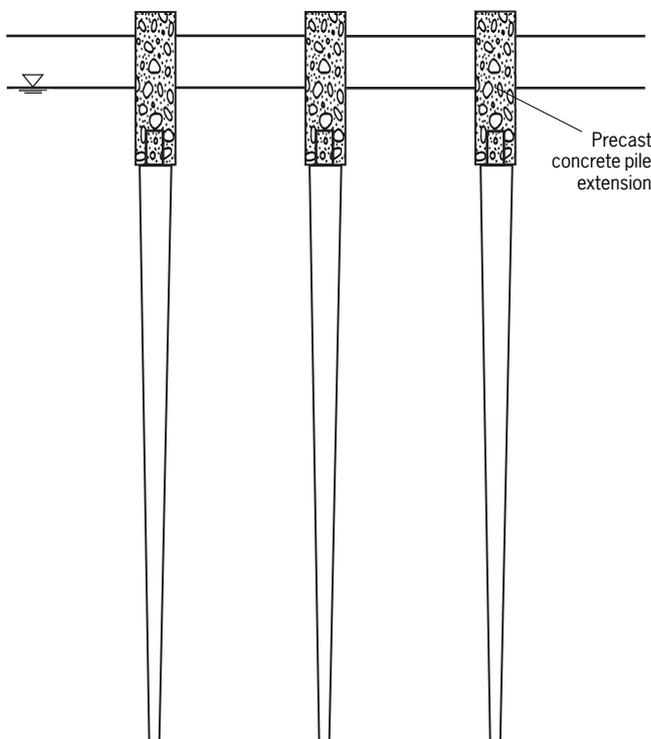
**Figure 2** Tapered untreated timber friction piles
