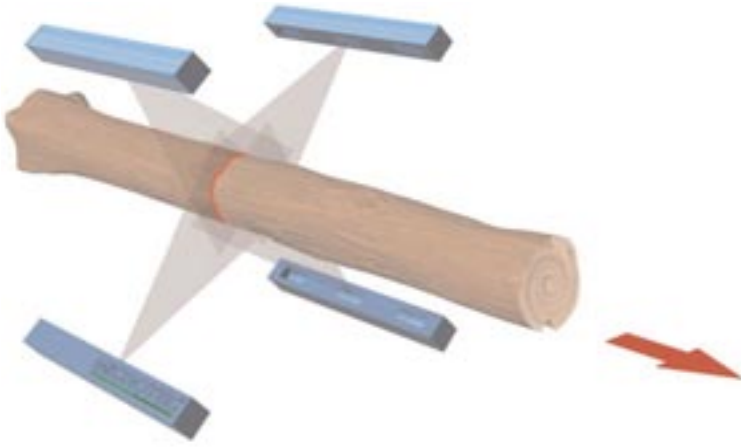
Figure 1 3D log shape scanner based on laser sheet-of-light triangulation (Image courtesy of Microtec)
