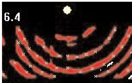
Figure 3 Screenshot of BRE developed software showing rate of growth and pith prediction. The white dot is the predicted pith position
