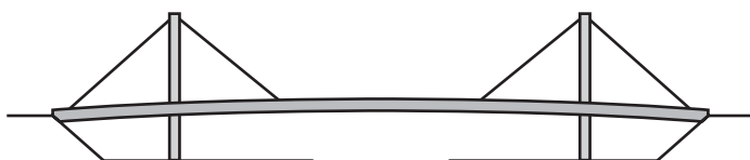
Figure 14 Cable stayed bridge
