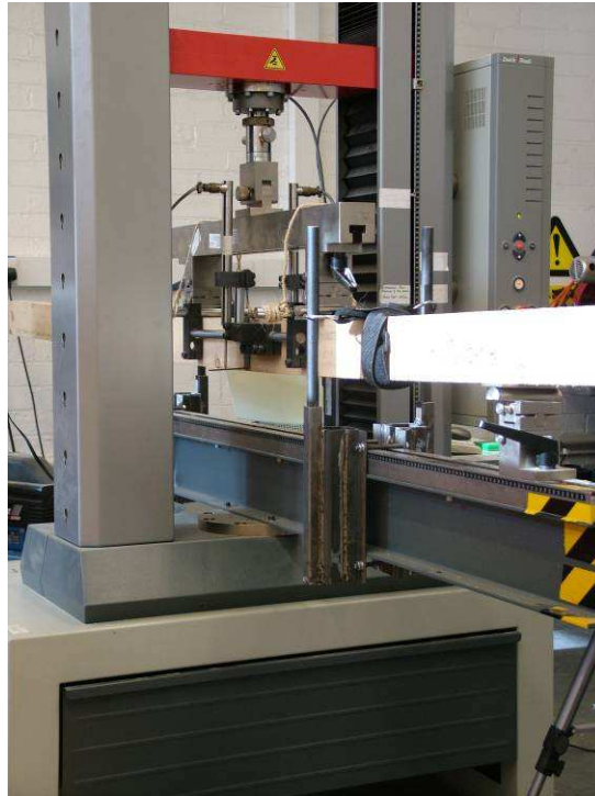
Figure 1. Four-point bending test conducted using the Zwick Z050 universal testing machine.
