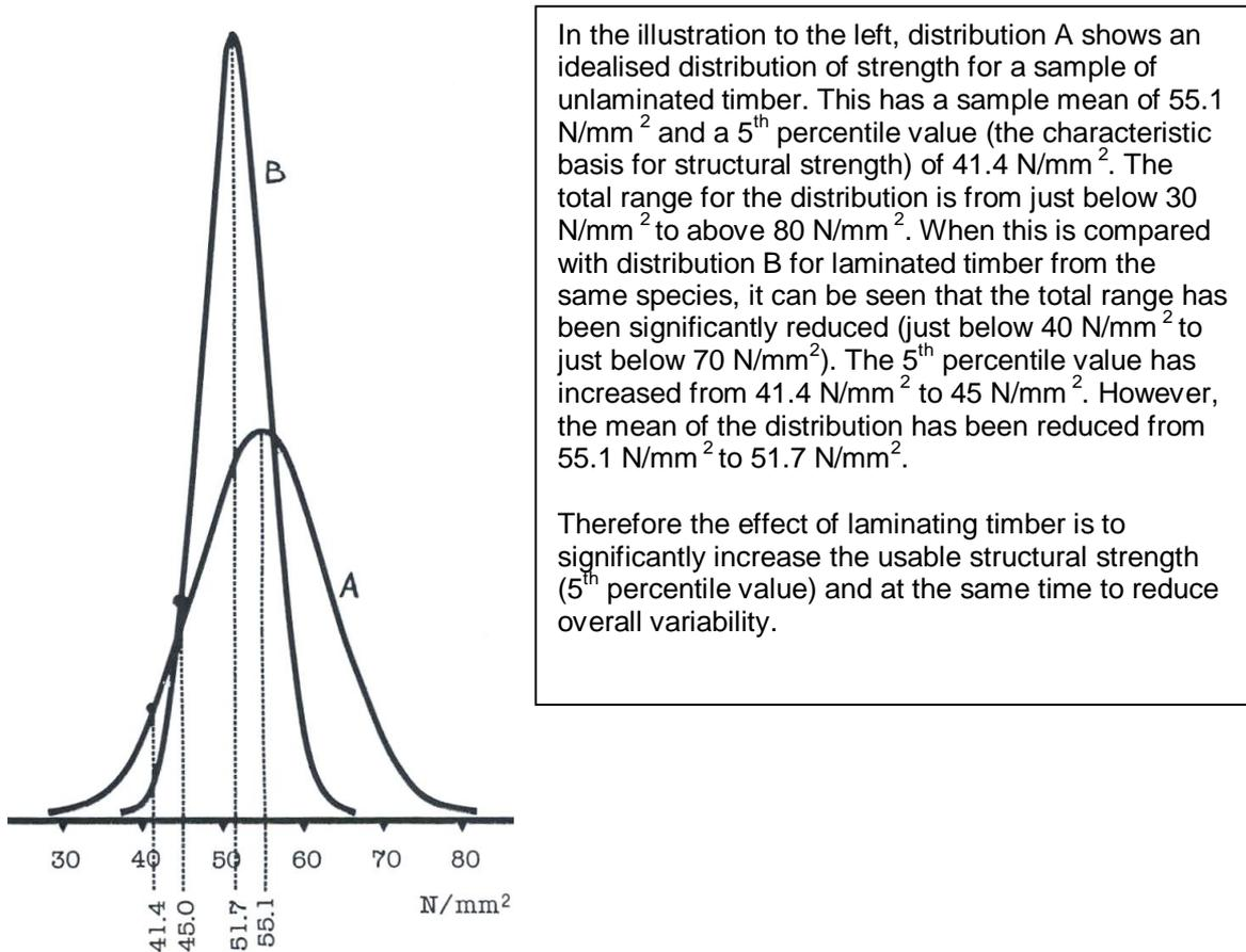
Figure 1 Illustration of the effect reduced variation has upon laminated strength
