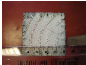
Figure 1: showing spikes of preservative penetration with little lateral penetration
