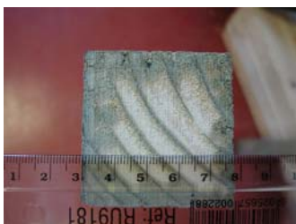
Figure 2: showing lateral penetration from incisions and an effective protective envelope treatment.
