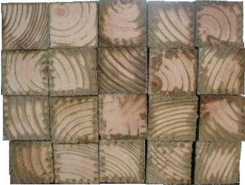
Picture 13 Preservation treatment HP4, showing better lateral penetration of preservative with development of some protective envelopes.
