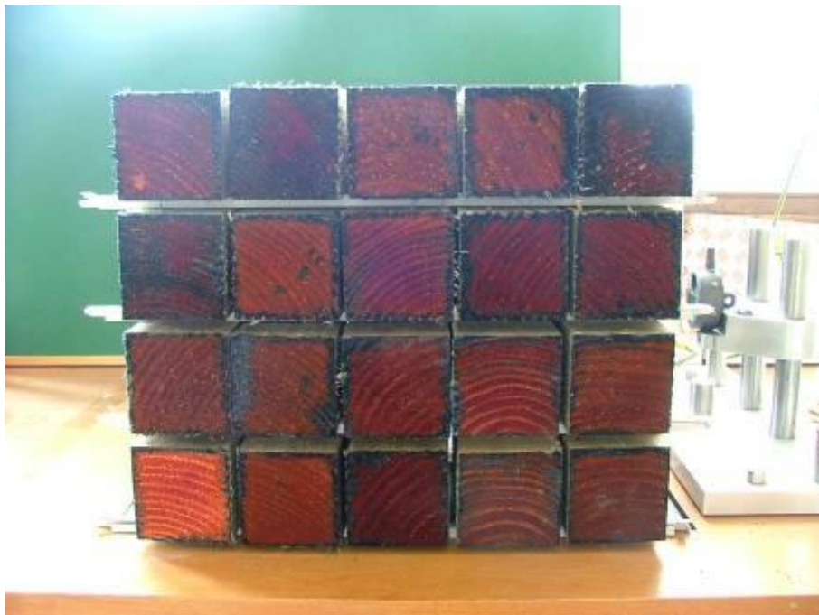
Figure 8: Visual assessment of samples treated using schedule 2 with 2.74% Tanalith E
