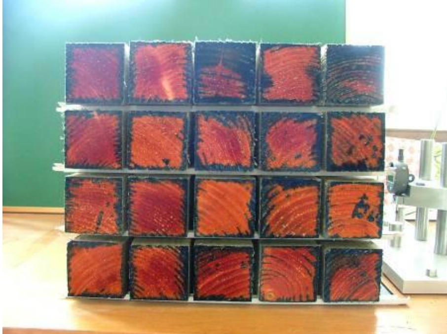
Figure 7: Visual assessment of samples treated using schedule 1 with 2.74% Tanalith E
