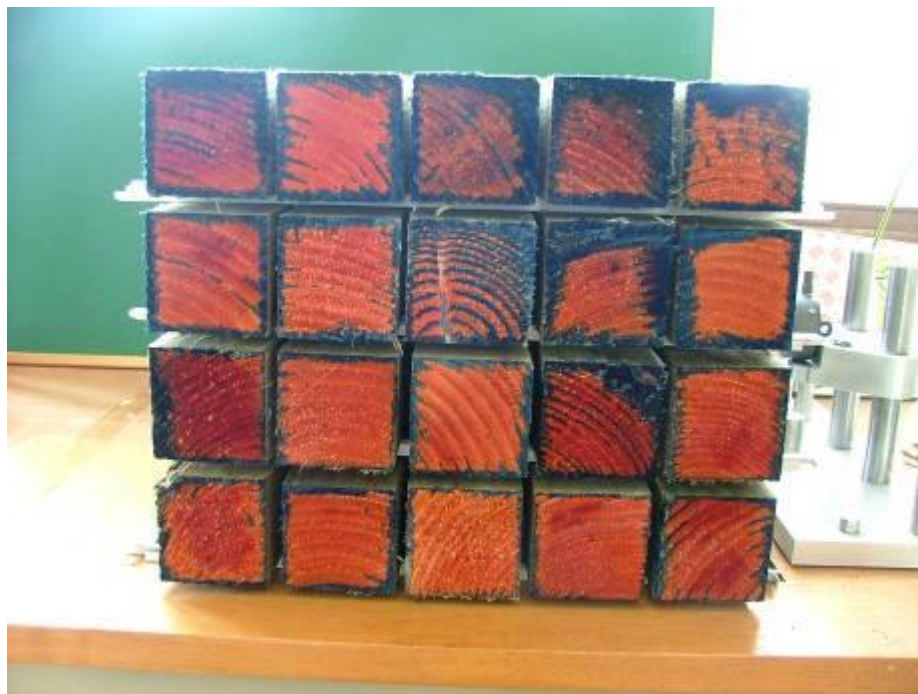
Figure 9: Visual assessment of samples treated using schedule 2 with 4.57% Tanalith E.
