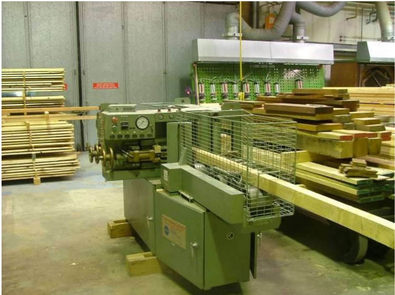
Figure 5: Apparatus used for pilot scale incising.
