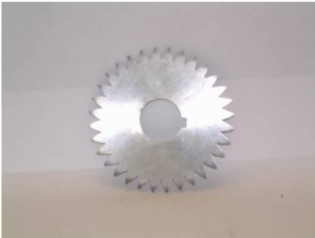
Figure 2: New incising blade pattern used in BRE trials.
