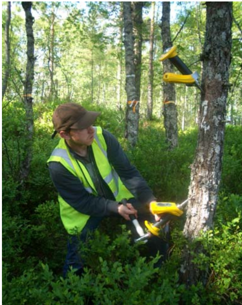
Fig. 1: Acoustic assessment of naturally regenerated Scots pine with the Director ST300, Glengarry, June '06.
