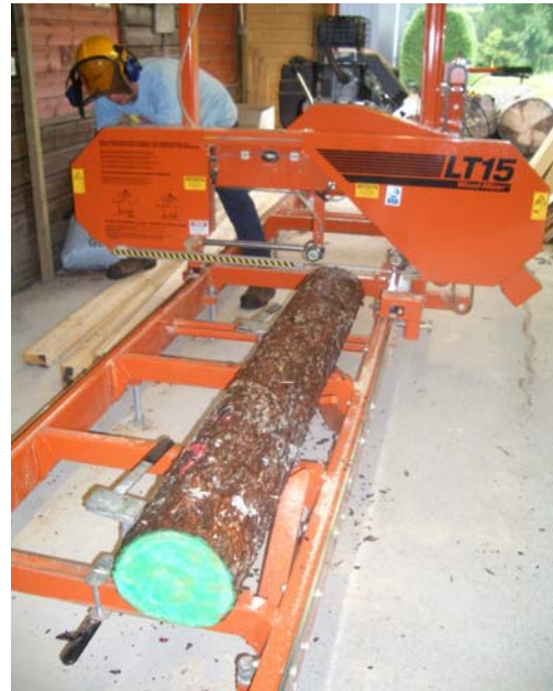
Fig. 2: Cutting of logs for small clears using Wood-Mizer saw. June, '06.
