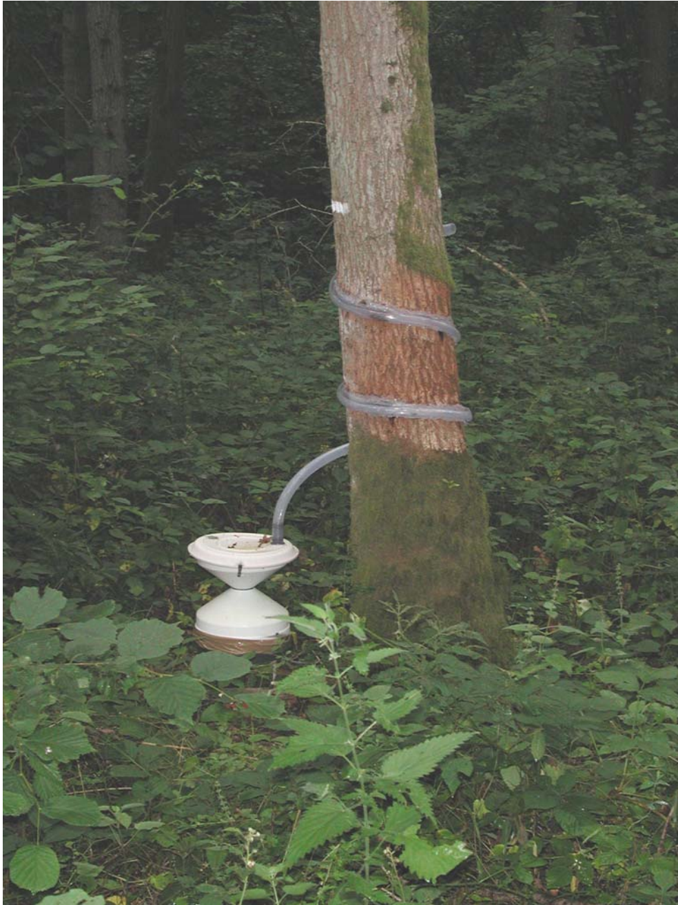
Plate 3: Automated Stemflow Collector (July 2003)
