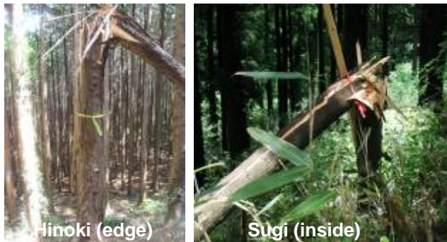
Figure 3: Ruptured sugi and hinoki in the tree-pulling experiments in Chichibu & Kamiatago
