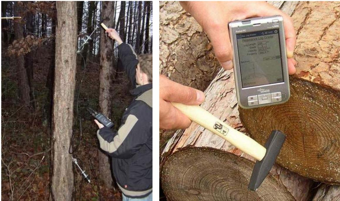
**Figure 2: Fakopp Instruments acoustic tools for measuring timber stiffness in standing trees (left) and logs (right)**
