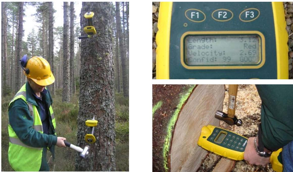
Figure 1: Fibre-Gen acoustic tools for measuring timber stiffness in standing trees (left) and logs (right)
