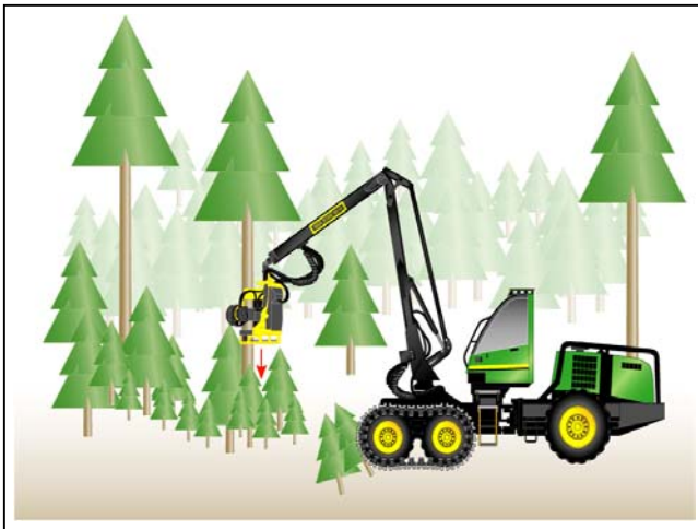
Figure 3 Placing the felling head high up the stem and running the rollers down to the base to aid head location for felling
