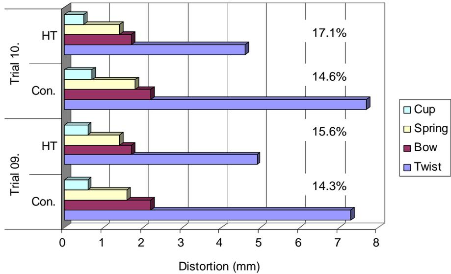
Figure 5. Average distortion & M/C values for experimental and control trials 09 & 10
