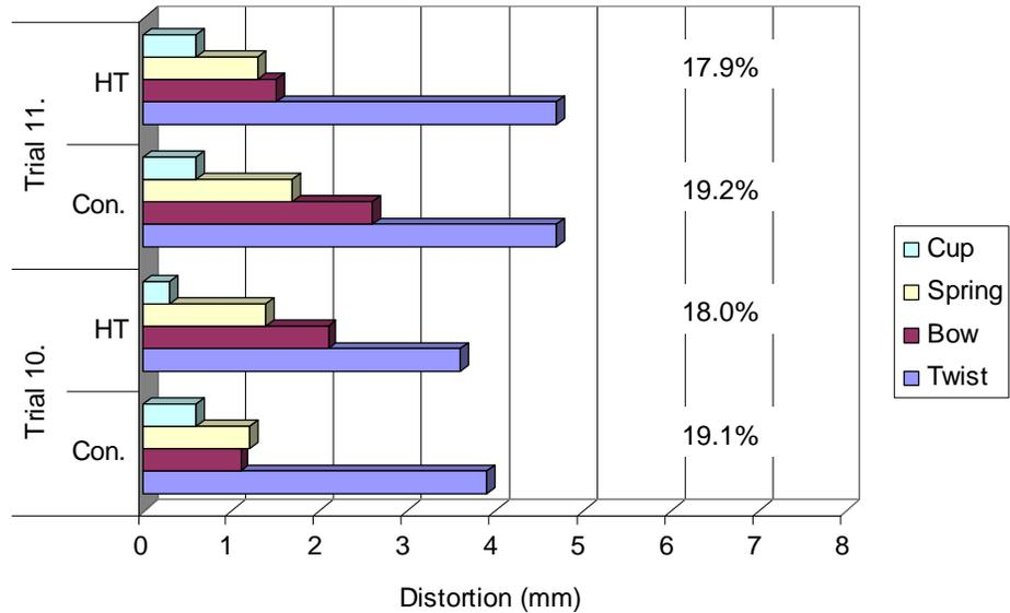
Figure 6. Average distortion & M/C values for experimental and control trials 11 & 12
