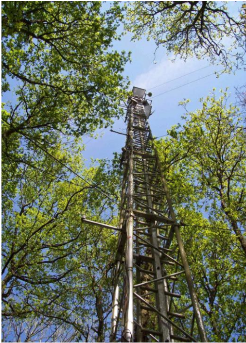
The flux tower at Alice Holt Forest monitors the exchange of carbon dioxide between the atmosphere and forest.
