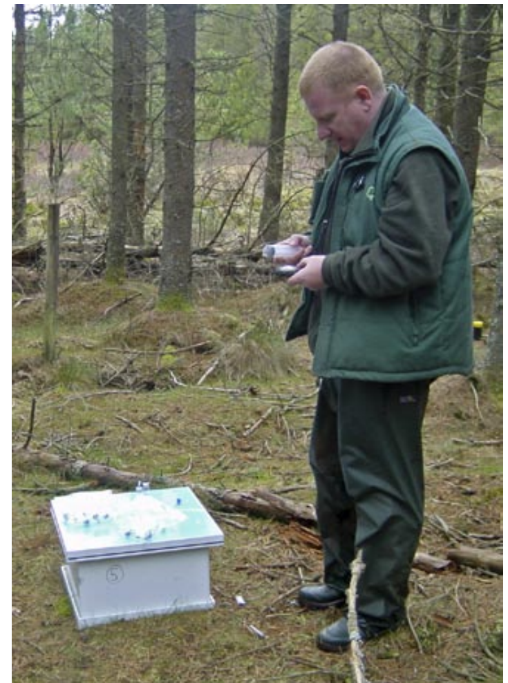
Sampling of greenhouse gases using a closed flux chamber at the Flanders Moss peatbog site in Sterling
