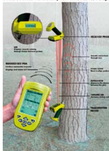
Figure 4: Time-of-flight method: Here we measure the speed of sound directly in the outer 2-3cm of wood in the standing tree.
