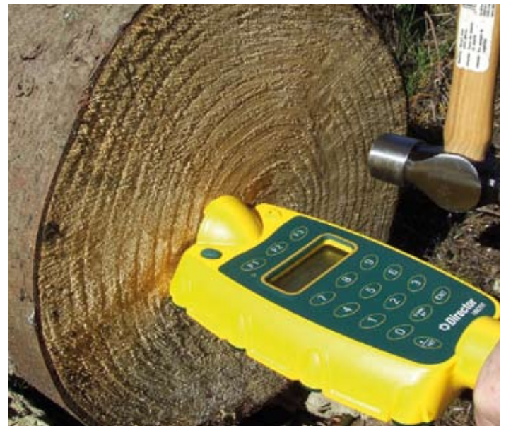
Figure 2: Acoustic tools can help increase efficiency in forest industries by allowing us to segregate poor quality material before processing
