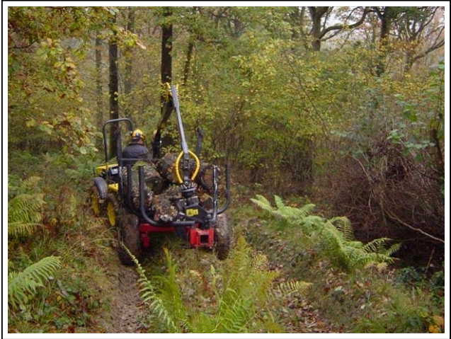
Figure 2 Narrow dimensions allow access on narrow tracks with minimal disturbance to trackside vegetation
