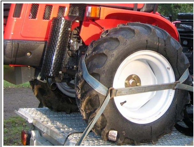
Figure 10 Tractor exhaust mounted in a position vulnerable to damage, next to the engine compartment
