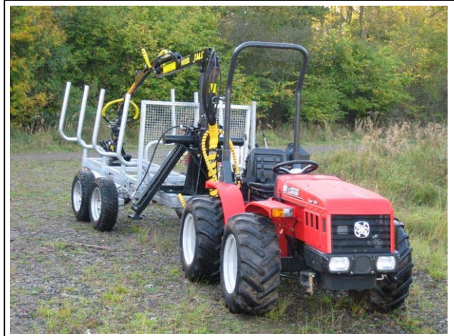
Figure 1 Small-scale alpine tractor and purpose-built forwarding trailer
