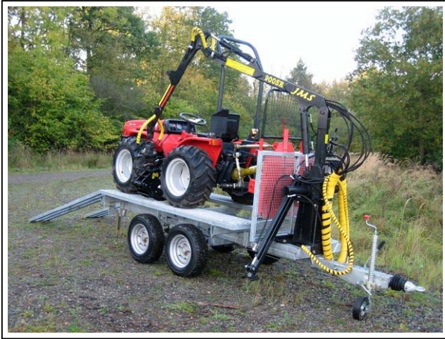
Figure 3 Transport to the forest worksite on a dual purpose trailer that can be converted into a forwarding trailer for use in the forest
