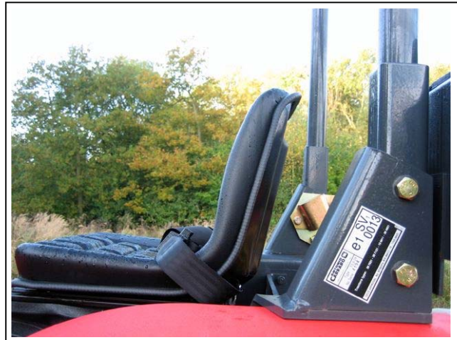
Figure 4 ROPS frame showing metal the plate stating the protection standard conformance. The lap restraint is also visible.
