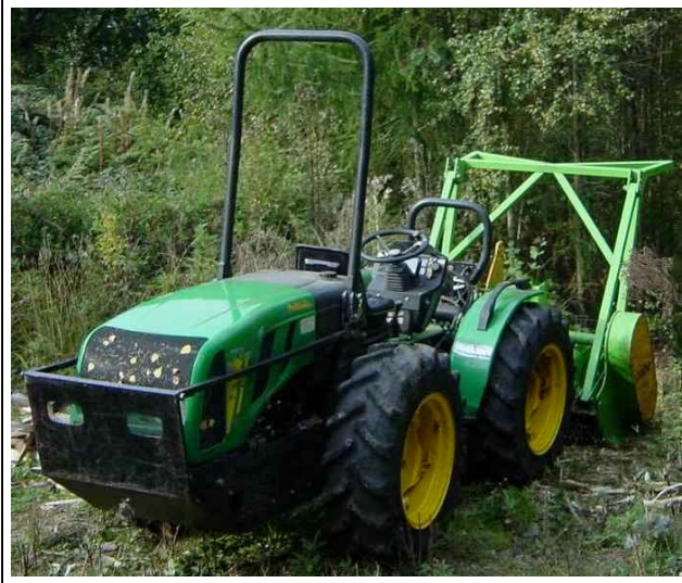
Figure 9 Guarding around the engine box and underbelly of a tractor attached to a mechanised flail
