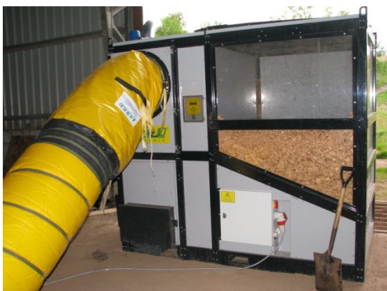
Lasco LA150 hot air boiler and flexible pipe
