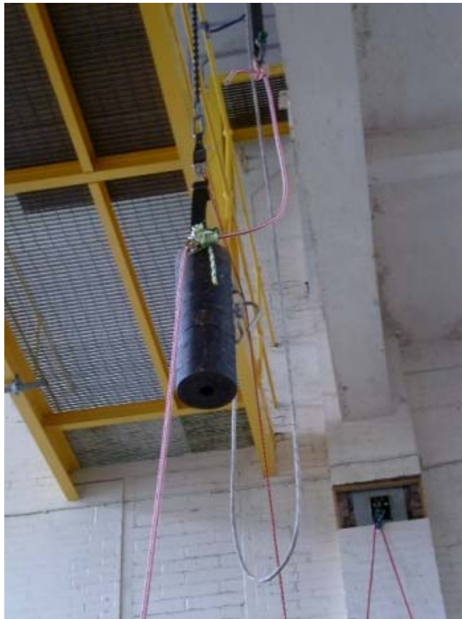
Photograph 12 The single rope drop test rig
