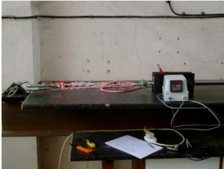
Photograph 11 The doubled rope pull test rig
