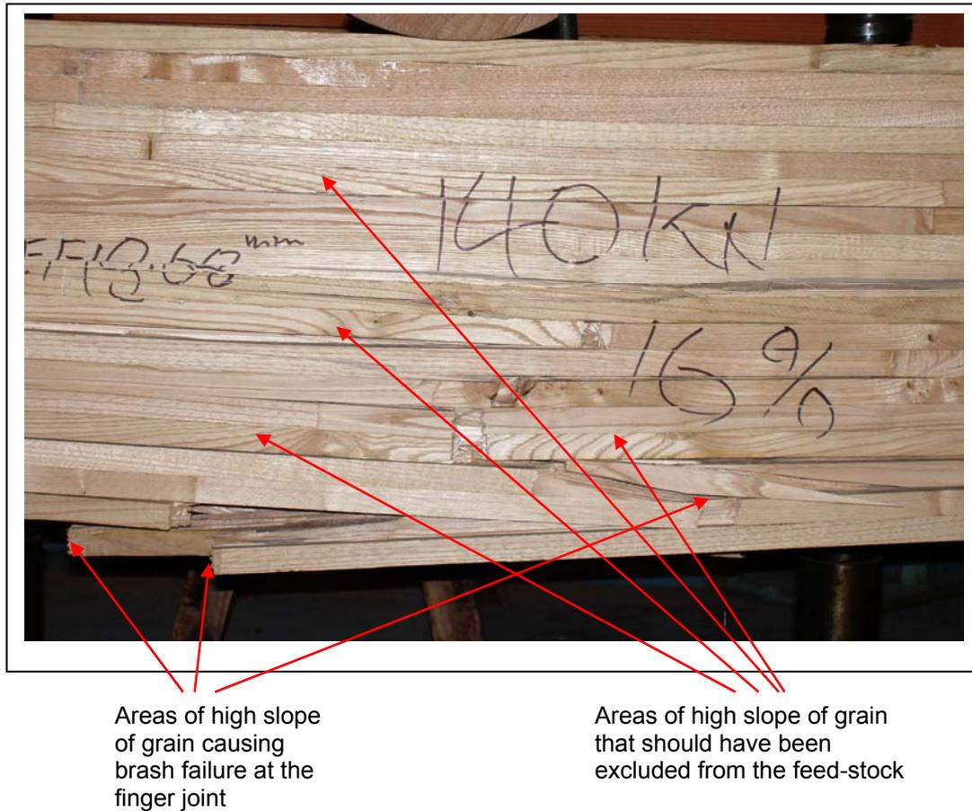
Figure 3. Showing areas of high slope of grain that should not have been included in the sweet chestnut beam and the effects upon performance.
