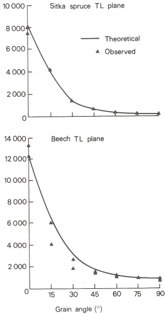
Figure 2. Effects of slope of grain upon stiffness (N/mm<sup>2</sup>)
