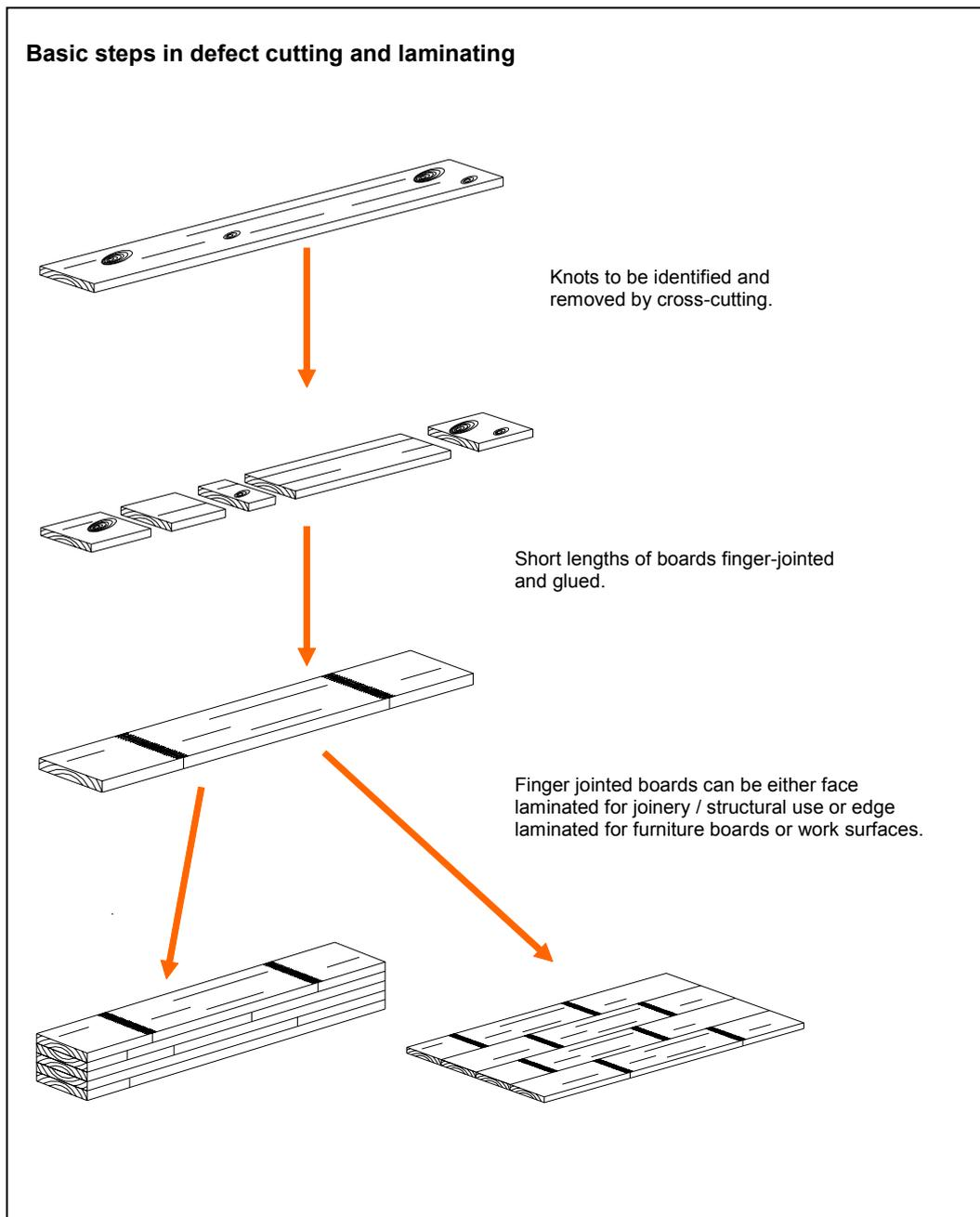
Figure 1. Steps in defect cutting and laminating
