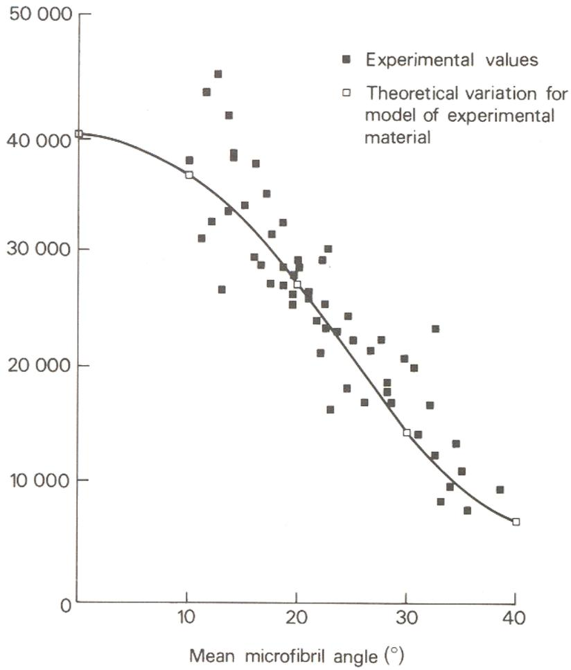
Figure 1. Effects of micro-fibril angle upon stiffness (N/mm<sup>2</sup>)
