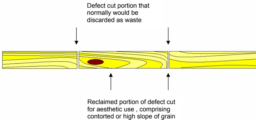
Figure 5. Shows the portion of defect cut material that can be reclaimed that has application for decorative use.
