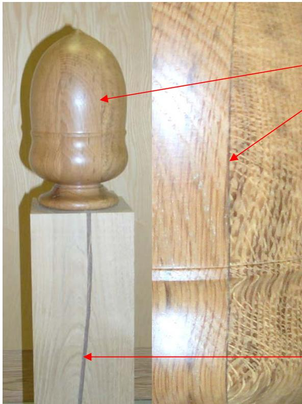
Drying stress degrade of the laminated oak acorn, slight peeling of surface fibres down one of the glue lines, the rest remaining intact. (Turning block originally 180mm x 180mm x 450mm )
