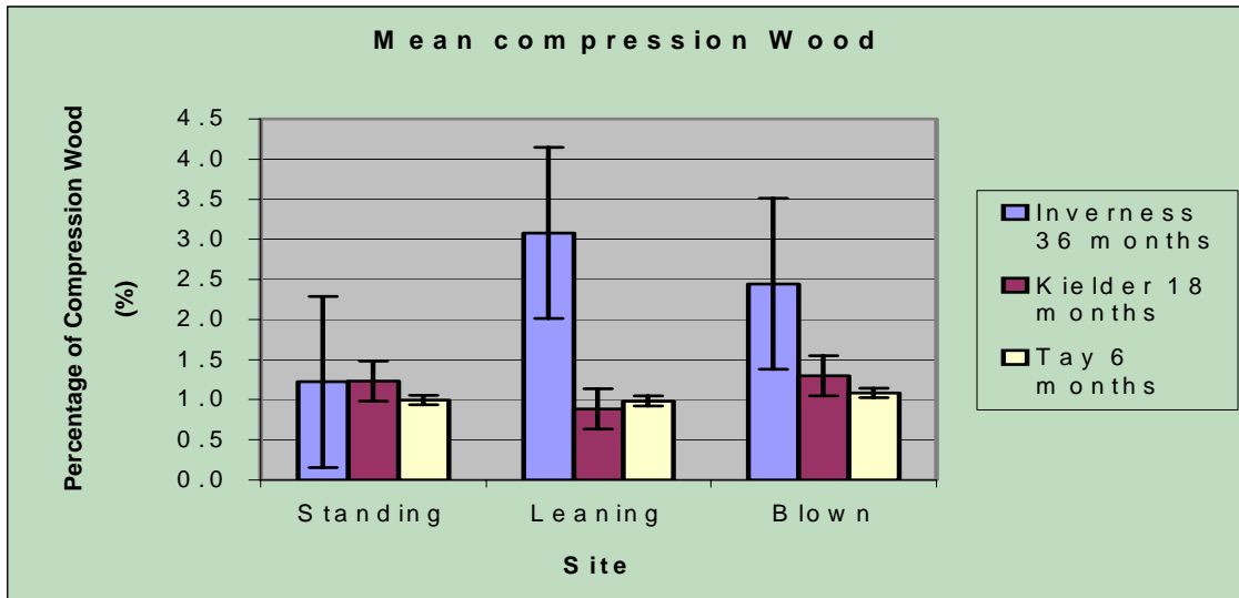
Figure 9- Mean percentage of compression wood as function of time since wind damage.
