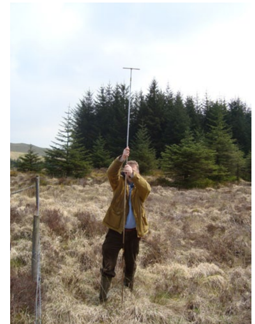
Measuring peat depth as part of the Field Assessment tool.
