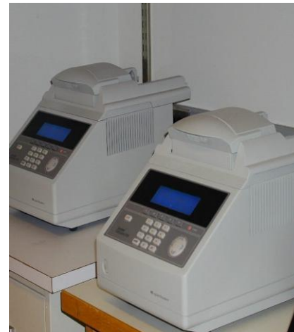
The Thermocyclers – the device enabling PCR
