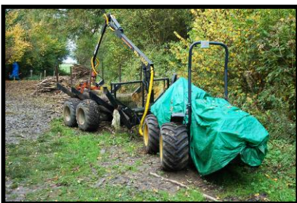
Left: tractor trailer forwarding of woodfuel arising from coppice restoration working BRADFIELD WOODS Right: processing of woodfuel arising from coppice restoration working
