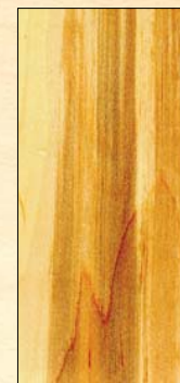
Staining of Hard maple (Discolouration during storage)
