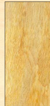
Oxidative staining of Framiré (Discolouration during kiln-drying)
