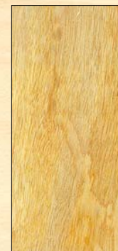
Oxidative staining of Framiré (Discolouration during kiln-drying)
