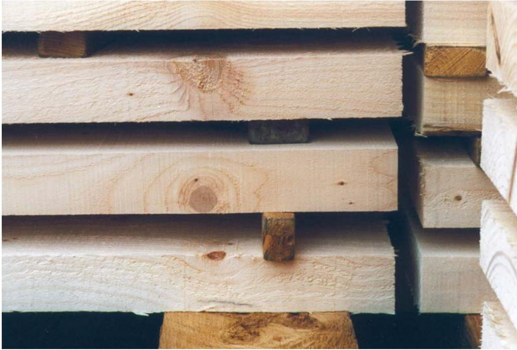
Figure 2a. Incorrect Sticker Alignment & Placement
