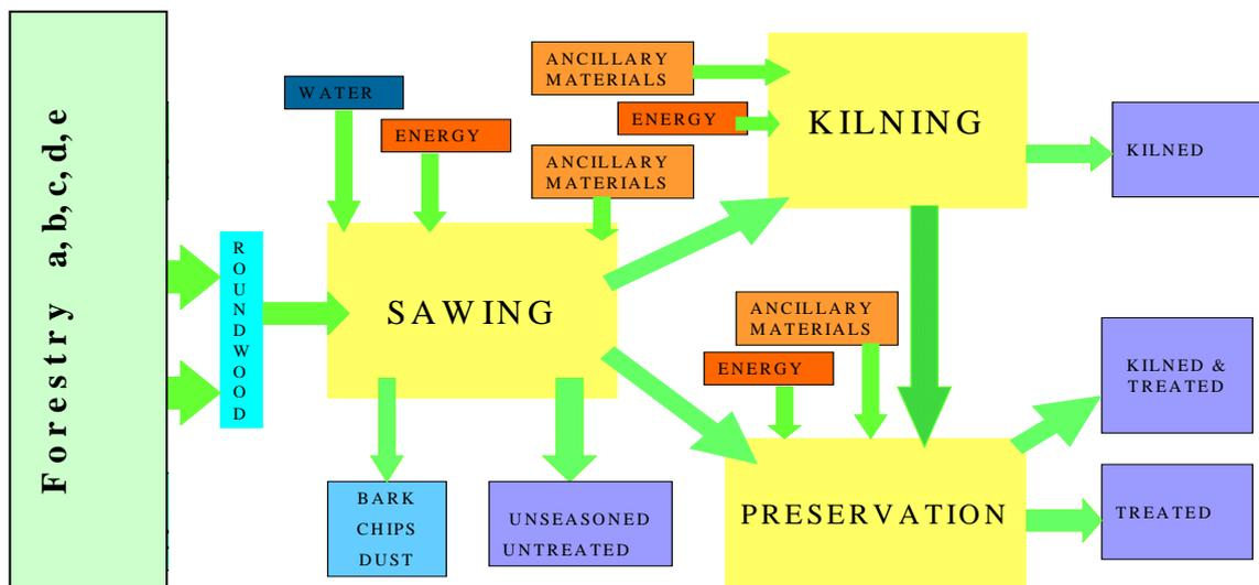
Figure 2: Generic process flow diagram for sawmilling
