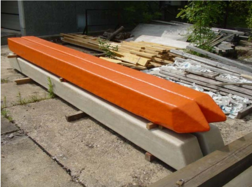
**Figure 1: Experimental FRP coated Douglas fir pilings (4.8m long x 250mm sq.)**
