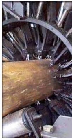
**Figure 1.** Groundline incising for processing utility poles.
