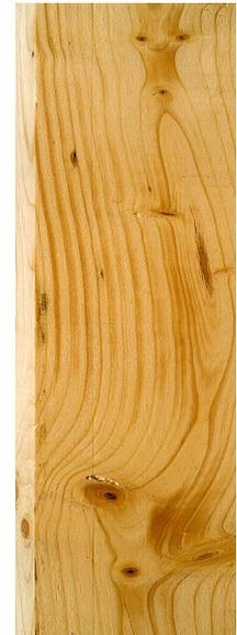
The detection of severe slope of grain was studied by using a specific sample of reject grade material. It was concluded, not surprisingly, that  $E_{dyn}$  based methods can hardly detect such defects. Old static bending type machine is quite effective in this respect. A clear need for grading method which can detect large grain angles was identified.
