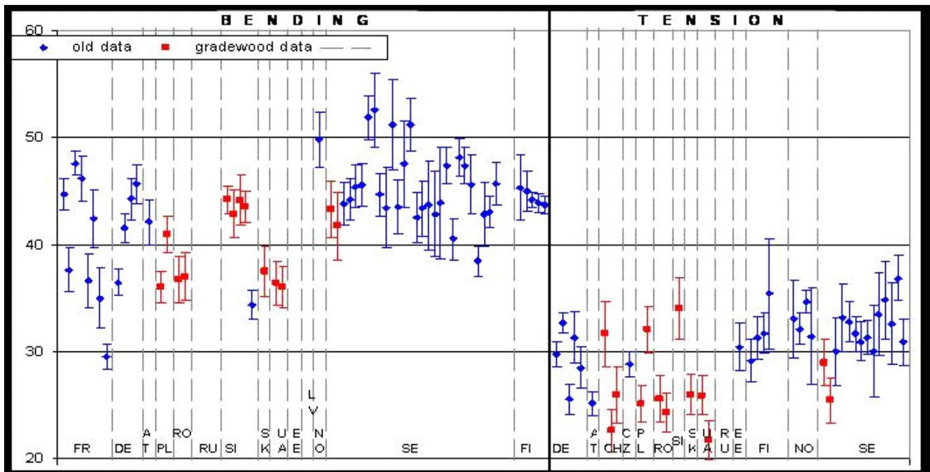
Figure 3. Variability of bending and tension strength of spruce of samples.
