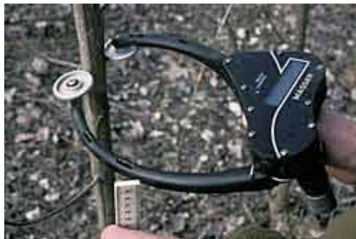
Measuring SRC stem diameters using Masser callipers
