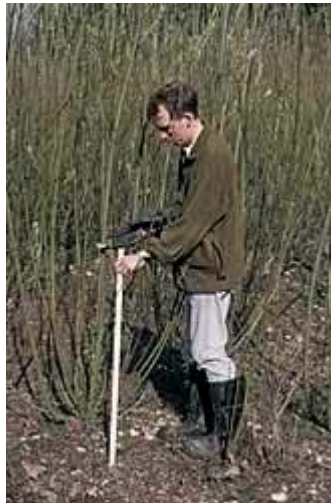
Measuring SRC stem diameters using Masser callipers
