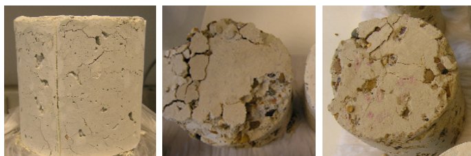
Figure 8. Damage on stabilised/solidified soil samples following different imposed climate scenarios.
