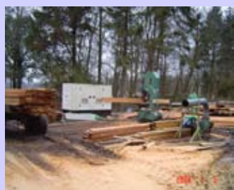
Forester resawing WRC into weatherboard
