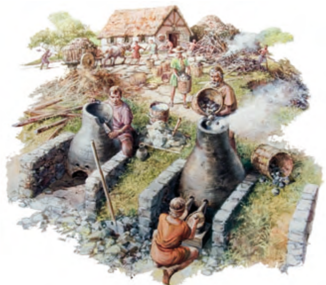
Artist's reconstruction of a Roman bloomery for iron production (reproduced with the kind permission of the High Weald AONB)
